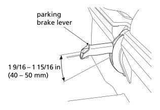
If adjustment is necessary, have the parking brake adjusted by your dealer.
