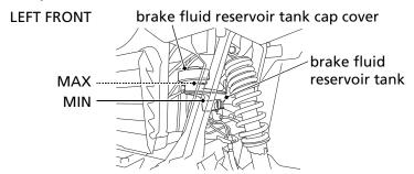
It should be between the MIN and MAX level marks. If the level is at or below the MIN level mark, check the brake pads for wear (page 157).
