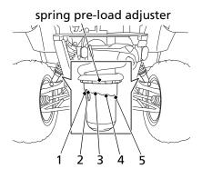
The spring pre-load adjuster has 5 positions for different load or driving conditions. Before adjusting the spring pre-load, jack up your Honda SXS (page 110) to avoid damaging the adjusters.
