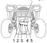
The spring pre-load adjuster has 5 positions for different load or driving conditions. Before adjusting the spring pre-load, jack up your Honda SXS (page 110) to avoid damaging the adjusters.
