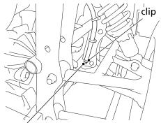
air cleaner housing drain tube plug
