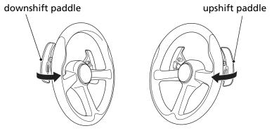
The transmission cannot be upshifted from neutral to D gear when the engine speed is above 3,000 rpm or the ground speed is above 2 mph (3 km/h) or the accelerator pedal is pressed.
