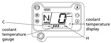
If all sections of the coolant temperature gauge, including segment H and high coolant temperature indicator are on (automatically appears in the display), stop the engine and check the reserve tank coolant level. Read page 202 and do not drive the SXS until the problem has been corrected.
