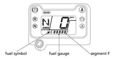
Regardless of what mode the display is in, when the fuel level reaches only one segment remaining, the display will automatically switch to the fuel gauge display. You should refuel as soon as possible.
