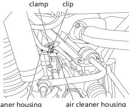
air cleaner housing drain tube
