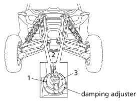
The damping adjuster has 3 positions for different load or driving conditions.
