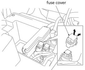
brake traction control system (BTCS) fuse
