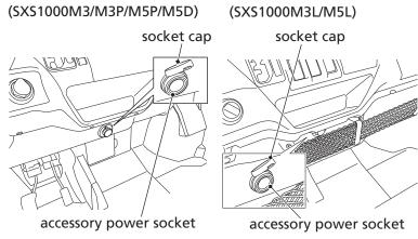
To use the accessory power socket, the engine must be running.
