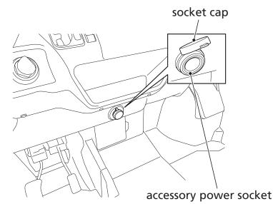
To use the accessory power socket, the engine must be on and idling.
