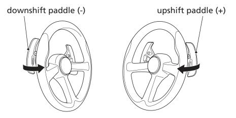
Pull the upshift paddle (+) to shift to a higher gear position and the downshift paddle (-) to shift to a lower gear position.
