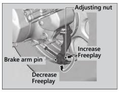
Apply the brake several times and check for free wheel rotation after the brake lever is released. **3.** Push the brake arm to confirm that there is a gap between the rear brake adjusting nut and brake arm pin.
