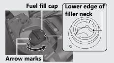
Do not fill with fuel above the lower edge of the filler neck.
