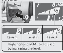
The selected level is maintained even when the ignition switch is turned to the OFF position, or transmission is switched to out of S mode.
