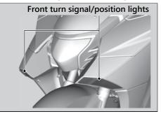
The front turn signal/position lights use several LEDs.
