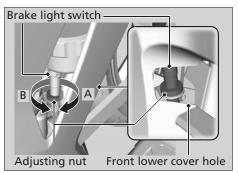
Check the operation of the brake light switch.
