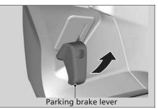
Place your motorcycle on a firm, level surface. Stop the engine and push your motorcycle while applying the parking brake lever to check the efficacy of the parking brake.
