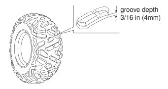
To check the condition of a tire tread, measure the groove depth in the center of the tire.
