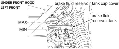
It should be between the MIN and MAX level marks. If the level is at or below the MIN level mark, check the brake pads for wear (page 142).
