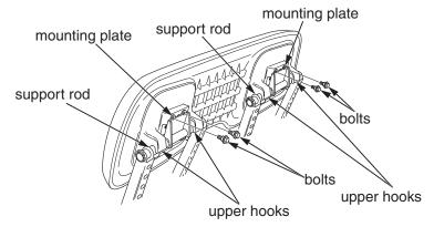
To return the seat-back to a more rearward position, follow the general instructions above, setting the lower hooks on the support rod and using the lower bolt holes.
