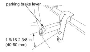
If adjustment is necessary, have the parking brake adjusted by your dealer.
