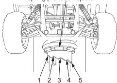
The spring pre-load adjuster has 5 positions for different load or riding conditions. Before adjusting the spring pre-load, jack up your Honda MUV (page 94) to avoid damaging the adjusters.
