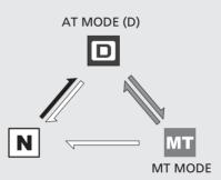
**Neutral (N):** Neutral is selected automatically when you turn the ignition switch to ON.
