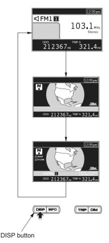
If you are not in the Navigation System when you turn the ignition switch OFF, you will see the audio display when you turn the ignition switch ON again. If you were in the system, you will see the system disclaimer with ENT highlighted.
