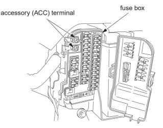
For your convenience, your motorcycle is equipped with an accessory (ACC) terminal and optional accessory socket. The terminal and socket provide 12V DC power for electrical accessories. When both terminal and socket are being used, the combined power rating of each accessory should be 60 watts (5 amps) or less. Before installing any accessories, read *Accessories & Modifications*, page 4.
