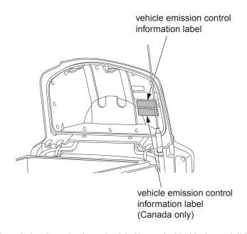
The Vehicle Emission Control Information label is attached inside the trunk lid.
