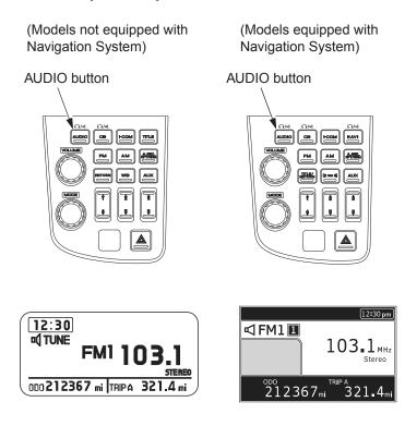
To turn the audio system off – push and hold the AUDIO button.
