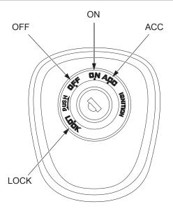
The ignition switch is used for starting and stopping the engine (page 71) and to lock the steering for theft prevention (page 87). Insert the key and turn it to the right for the ON and ACC (accessory) positions.
