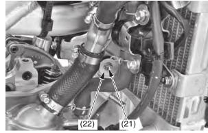
(21) right radiator lower mounting bolt (22) washer
