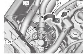
(7) clamp (8) bolt (9) clamp tab (10) groove
