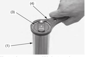
(1) outer tube(3) fork damper assembly
