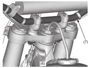
(6) handlebar lower holder nuts, washers and mounting rubbers(7) handlebar
