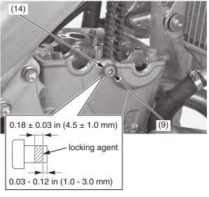
(9) sealing bolt(14) sealing washer (new)
