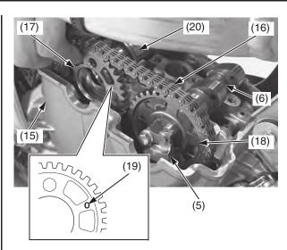
(5) decompressor weight(6) exhaust camshaft(15) cylinder head(16) cam chain
