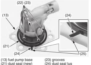
(24) dust seal lu (25) index mark 9. Apply small amount of engine oil to a new O-ring (26).
