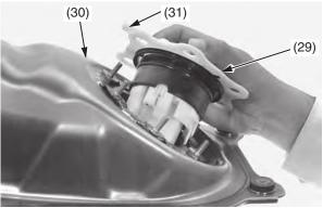
(29) fuel pump unit(30) fuel tank(31) hose joint
