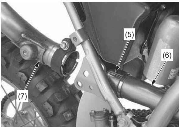
(5) gasket (new) (6) exhaust pipe (7) muffler
