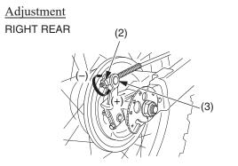
(2) rear brake adjusting nut(3) brake arm pin
