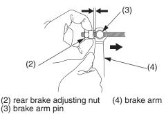
After adjustment, confirm the freeplay of the brake pedal.
