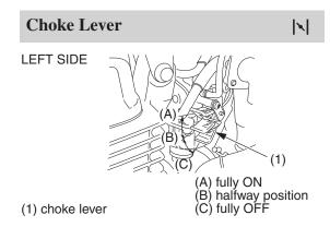
The choke lever (1) is used for starting the engine (page 29). The choke increases the percentage of fuel in the fuel/air mixture delivered to the engine.
