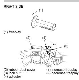
Inspection Check freeplay (1). Freeplay: 1/16–1/4 in (2–6 mm)
