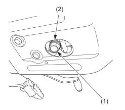
(1) oil drain bolt(2) sealing washer
