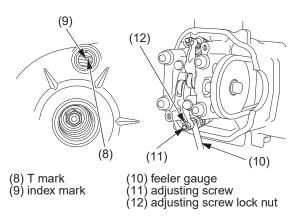
4. Rotate the generator flywheel counterclockwise until the T mark (8) on the flywheel lines up with the index mark (9) on the left crankcase cover. In this position, the piston may either be on the compression or exhaust stroke.
