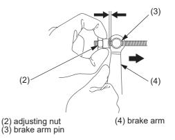
After adjustment, confirm the freeplay of the brake pedal.
