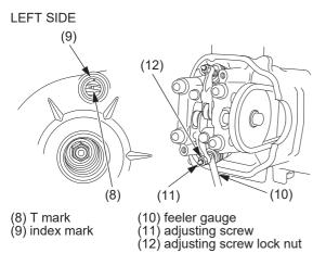
4. Rotate the generator flywheel counterclockwise until the T mark (8) on the flywheel lines up with the index mark (9) on the left crankcase cover. In this position, the piston may either be on the compression or exhaust stroke.
