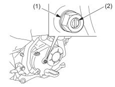
(1) adjuster lock nut(2) clutch adjuster
