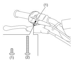
(1) M5x10 screw (2) M5x40 screw You can reduce throttle grip movement.
