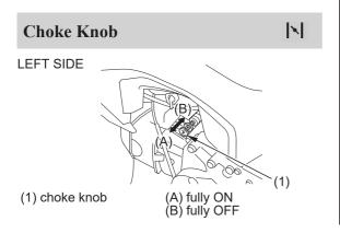
The choke knob (1) is used for starting the engine (page 32). The choke increases the percentage of fuel in the fuel/air mixture delivered to the engine.
