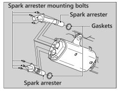
**5.** Use a brush to remove carbon deposits from the spark arrester screen. Be careful to avoid damaging the spark arrester screen. The spark arrester must be free of breaks and holes. Replace, if necessary. Check the gasket. Replace, if necessary.
