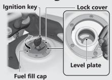
Do not fill with fuel above the level plate. Fuel type: Unleaded gasoline only
