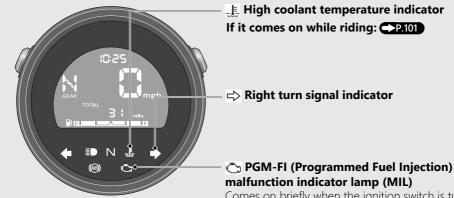
Comes on briefly when the ignition switch is turned to the ON position with the engine stop switch in the  $\bigcap$  (Run) position.
